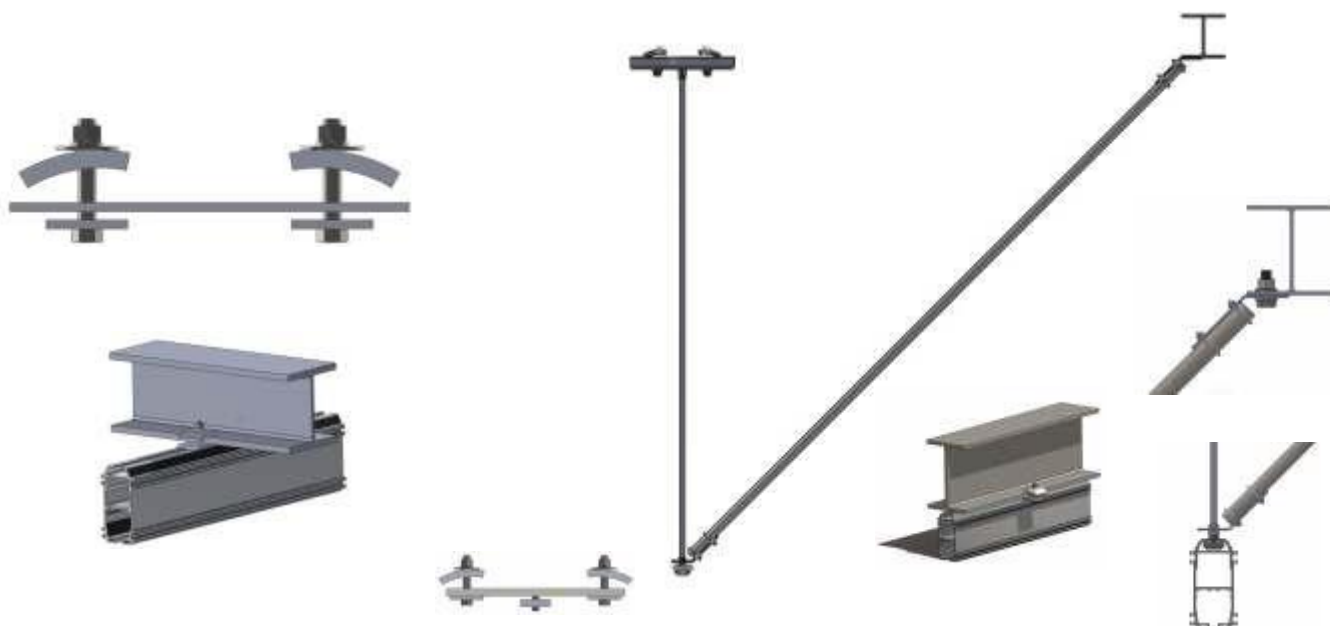
Type B with Sway Brace (Required for hangers over 24" in length.)
