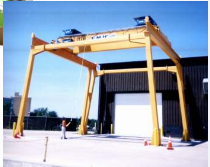
This freestanding 40/20 ton double girder crane handles protective concrete casings for telecommunication equipment.
