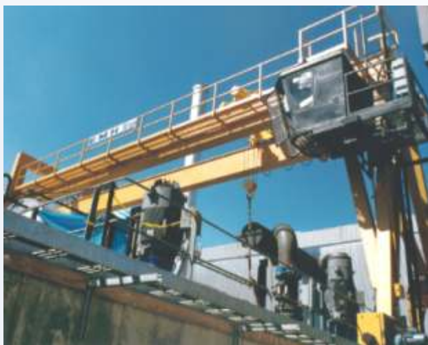
A rotating "hammerhead" hoist (inset) with 360 degree rotation allows smooth rotation of panels from inventory storage to truck loading.
