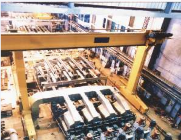
A double leg gantry with torsion box girder construction services roll stands in a continuous casting facility.
