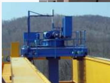
A 25 ton, 120 foot gantry (above) positions architectural concrete panels from production to storage..
